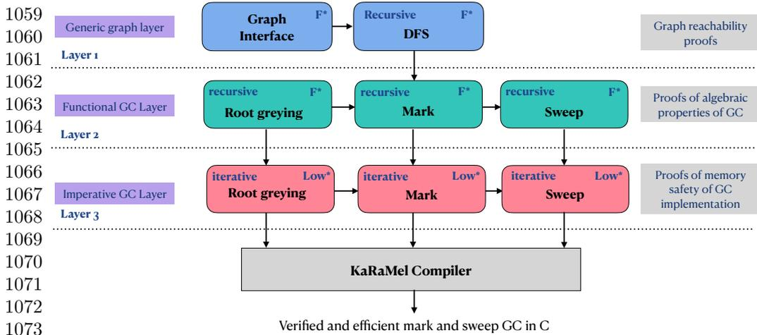
1075 **Fig. 18:** The layering approach for GC verification
