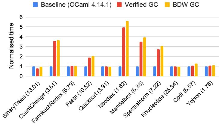
1808 **Fig. 29:** Normalized running time of different OCaml GCs. The numbers in the
