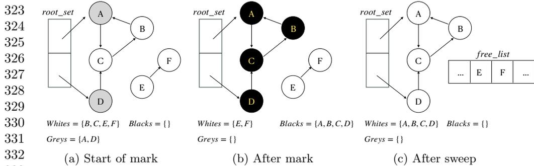
334 **Fig. 4:** Tricolor marking. Initially the objects that are directly pointed by the root
