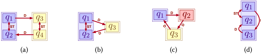
Fig. 12. Valid (a,b) and invalid (c,d) cycles where D \in \{WR, RW, WW\}
